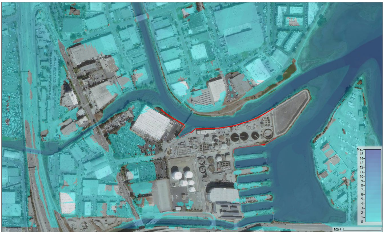
Figure 4-3. With-project floodwall alignments shown in red. Flood inundation displayed is resulting from an example tidal event with maximum elevation of 12.65 ft NAVD88.
